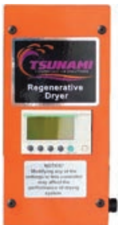
PROGRAMMABLE PLC CONTROLLER
