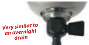
Semi-Automatic Drain (Poly Bowls only) Semi-Auto Drain releases moisture contents when less than 15 PSI is applied to bowl. (2000 & 8000 SERIES ONLY)
